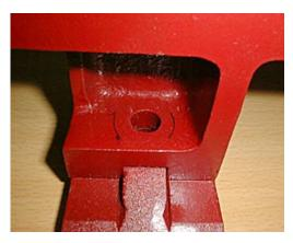
3. With the  $\frac{1}{2}$ " transfer punch, mark the back of the casting at the center of the hole through the cam lock sleeve.
