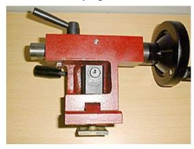
8. Put the tailstock back on the lathe and adjust the position of the clamping foot.
