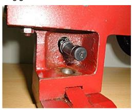
4. Assemble the cam lock socket and cam lock sleeve.
