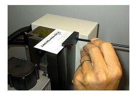
Do not install the Z-axis limit at this time. Later you need to move the head above the top of the column.
