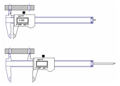
Be sure to use the same (inside) jaws for both measurements. And remember that this works only if the holes are the same size.
